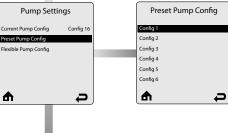
In the **Preset Pump Config.** (preferred selection) you can choose from a number of preset pump configurations. Only the configurations usable with a certain model/type of appliance will appear in the list. The configurations are detailed in Volume 2, "User's Guide". Each configuration is detailed through one or several hydraulic diagrams, a table indicating the electrical connections and a list of the parameters to be defined in ACVMax.
